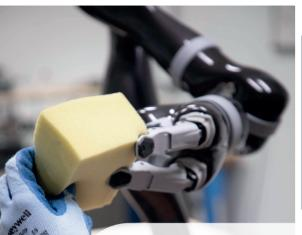
The manufacturing and processing of soft and flexible materials with varying shapes poses unique challenges to automation, such as requiring highly adaptable manipulation approaches.
